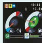
PM accumulation/ Urea accumulation display
