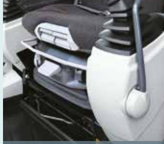
Seat suspension absorbs vibration
