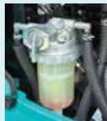
Pre fuel filter with built-in water separator
